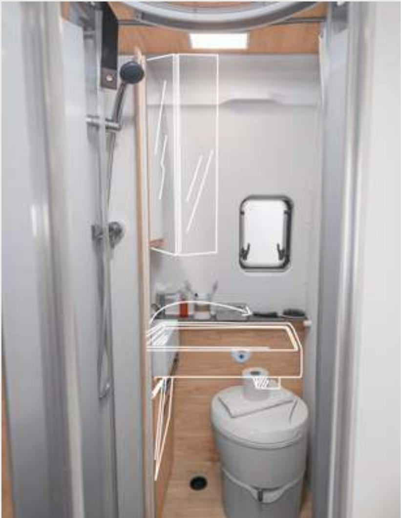
BOXDRIVE 680 ME. The spacious in-room bath is equipped with a retractable washbasin that – in a pulled-out version – has dimensions of up to 650 x 300 mm. Thanks to the hinged mirror, you can get a good look at yourself, even when the washbasin is folded out.
